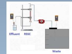
Figure 3: Continuous configuration of Rapid Small Scale Column Tests (RSSCTs)
