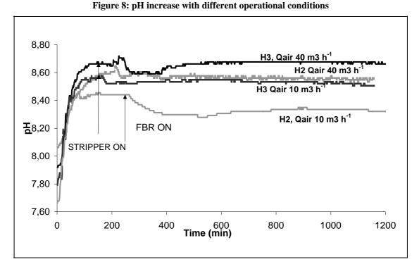
The pH highest value reached is 8.7, however lower than the one achievable using a typical anaerobic supernatant. This happens because of the low alkalinity value of the liquid used (1000 mgCaCO<sub>3</sub>/l).
