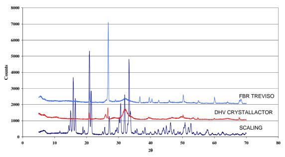
The same partially crystalline deposit was observed on nucleated material drawn from a DHV Crystallactor (Geestmerambacht, The Netherlands): in this case the deposit was mainly constituted by Ca and P salts (P salts to silica weight ratio 80/20). Finally, a complete crystalline scaling on diffuser device of Treviso FBR, was observed mainly formed by MAP and HAP or CP salts.
