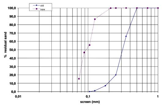
Figure 7: particle-size distribution from sieve analysis of sand particles
