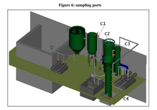
The first sample (C1) is taken from the mixer; this is the anaerobic liquor supplied from the press belt. Another sample, C2, is taken from the stripper and it represents the real feed (supernatants phosphate enriched). The C3 sample is taken from the de-aeration column bottom, and it represents the plant real effluent. The C4 sample represents the recycle flowrate.
