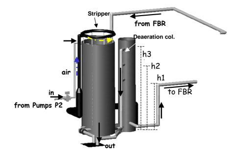
At the bottom of the stripper there is a valve for the tank cleaning; moreover the de-aeration column is connected to the stripper by means of an horizontal pipe. The liquid flows from the de-aeration column to the FBR through pump P1. The column has three outlets at three different heights (h1-h2-h3): depending on the selected height it is possible to set different volumes and, therefore, different operational conditions (i.e. hydraulic retention time).
