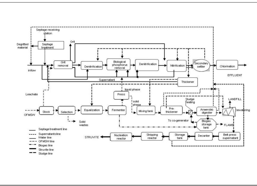
Fig.1: Treviso WWTP full logic flow
