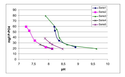
The figure shows two supersaturation curves (1 and 3) for higher pH, and two curves (2 and 4) for lower pH. At lower pH and higher P concentration precipitation of HAP (85-95%) and MAP (10-15%) occurs. When P content decreases, at higher pH, precipitation of calcite (60-80%), HAP(10-30%) and MAP(10-15%) takes place.
