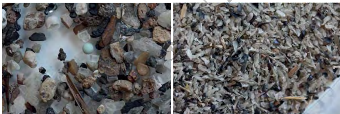
3236 Figure 2: Isolated impurities from (low-quality) struvite precipitate samples (adopted from 3237 STOWA, 2015). 3238 3239
