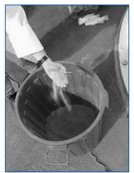
*Figure 1.* Photograph of MAP produced from the pilot-scale SC Process at the Oxley Creek wastewater treatment plant.
